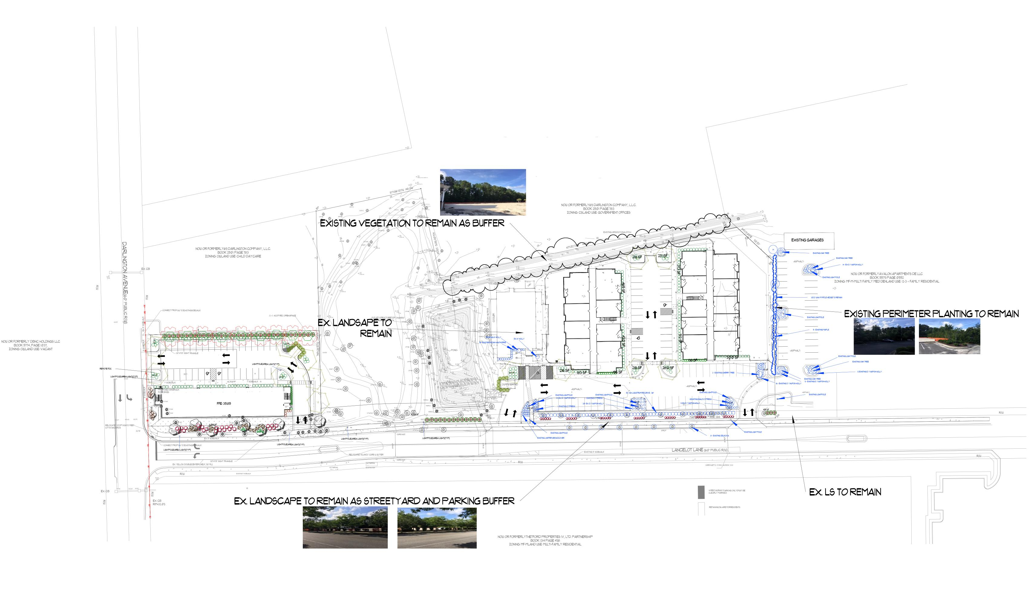
NOTE: PRIOR TO ANY CLEARING, GRADING, OR CONSTRUCTION ACTIVITY, TREE PROTECTION FENCING WILL BE INSTALLED AROUND PROTECTED TREES. NO CONSTRUCTION WORKERS, TOOLS, MATERIALS, OR VEHICLES ARE PERMITTED WITHIN TREE PROTECTION FENCING
